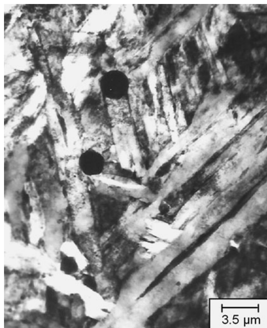
Fig. 10 TEM Photograph of weld metal M 21 revealing lath martensite and the acicular ferrite nucleated from inclusions
